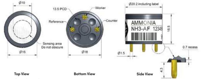
Dimensions are in millimetres (± 0.15 mm).
