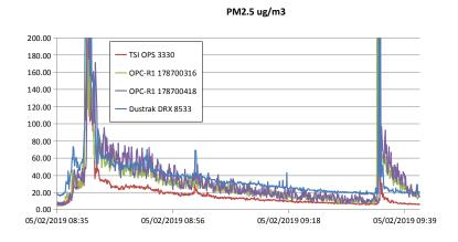
Figure 2 shows a comparison of PM2.5 monitoring by an OPCR series sensor and TSI OPS 3330 and DustTrak instruments. All are set at 5s averaging and are sampling the ambient air of a work shop, the raw 3330 data has been used to calculate a PM figure.
