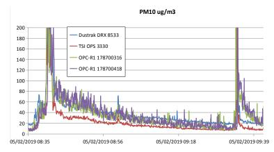
Figure 3 shows a comparison of PM10 monitoring by an OPCR series sensor and TSI OPS 3330 and DustTrak instruments.
