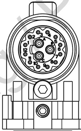
Matching pre-fabricated connection cables are available for the motors BG 45 dPro with a 12+3-pin connector. For detailed information, see chapter „[Connection via 15-pin connector for motor](#)“ on page 38.
