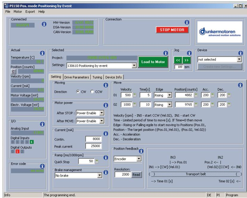
With the „Load to motor“ button, the user has the possibility of loading mode-specific parameter adjustments to the motor with the aid of the parameterising interface.
