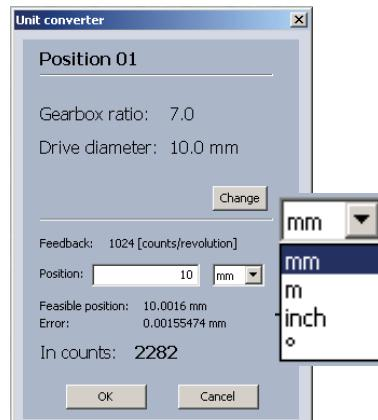
From the values gear ratio, shaft or wheel diameter, position and unit of measurement, the converter calculates the position in counts.
