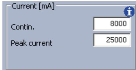
In this example, a continuous permissible phase current of 8 A and a peak current of 25 A are defined.
