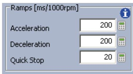
**Acceleration** allows the setting of the acceleration ramp.
