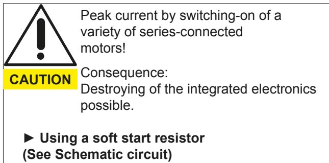
The inrush current must be realized by a soft start function when a variety of motors will be switched on. This is either possible by using of a adequate power supply unit or as shown in the schematic circuit.
