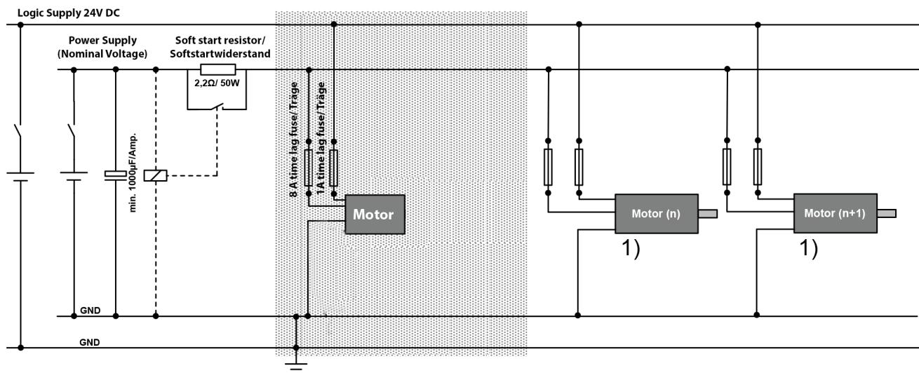
The grey section of the schematic circuit shows the connection of a BG65 PI. It is also possible to connect in series more BG-motors as shown.
