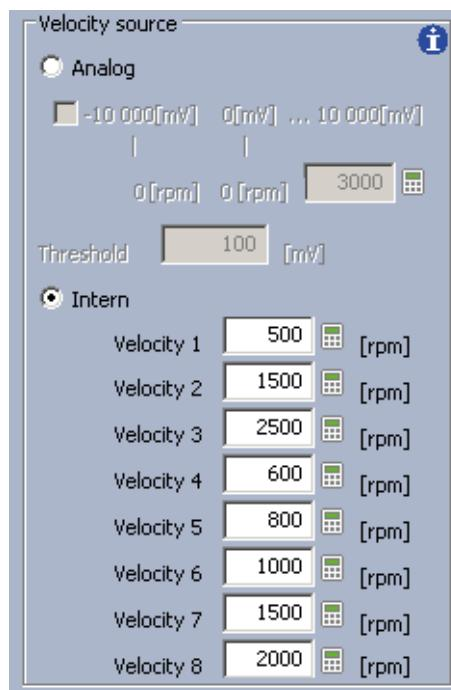
In this example, the velocities are activated via digital inputs.
