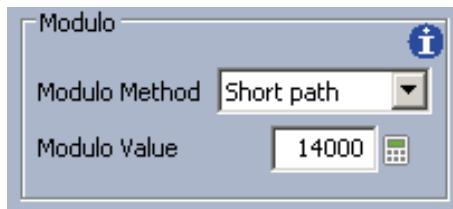
In this example, the motor will drive to the pending positioning by the shortest path. A full rotation was divided in 14000 steps.
