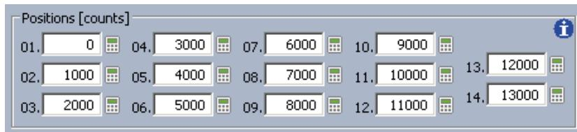
In this example, the identification number 01 is given a positioning with 0 counts.
