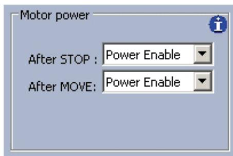
In this example, the position after a STOP will be held, however, after MOVE the motor is given freedom of movement.
