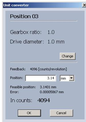
Enter in the input-fields the values for the gear ratio and the shaft diameter.
