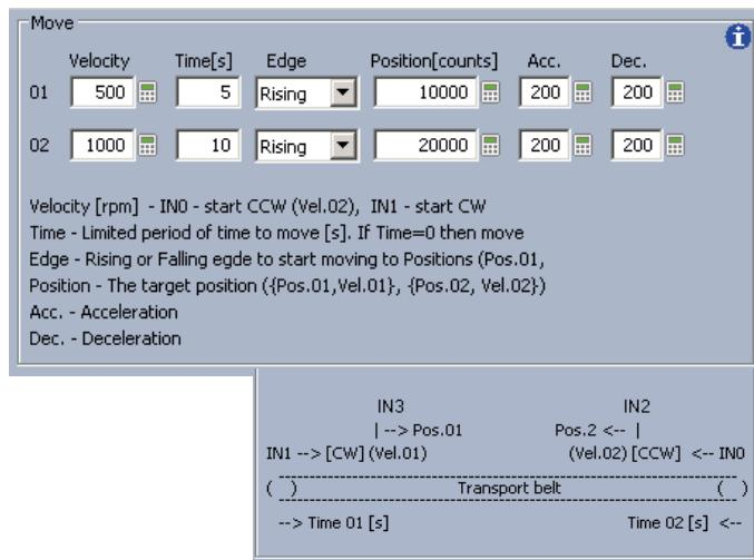
The parameter set divides itself into two driving sets. The first drive set is started by IN1 (CW), IN0 (CCW), and runs at defined speed for the defined time. This movement can be interrupted with the inputs IN2 (CCW), IN3 (CW) and can be looked with the movement defined under „Position“ (Positioning by Event).
