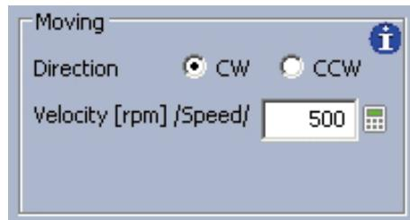
In this example, the motor runs at a speed of 500 rpm in the clockwise direction.
