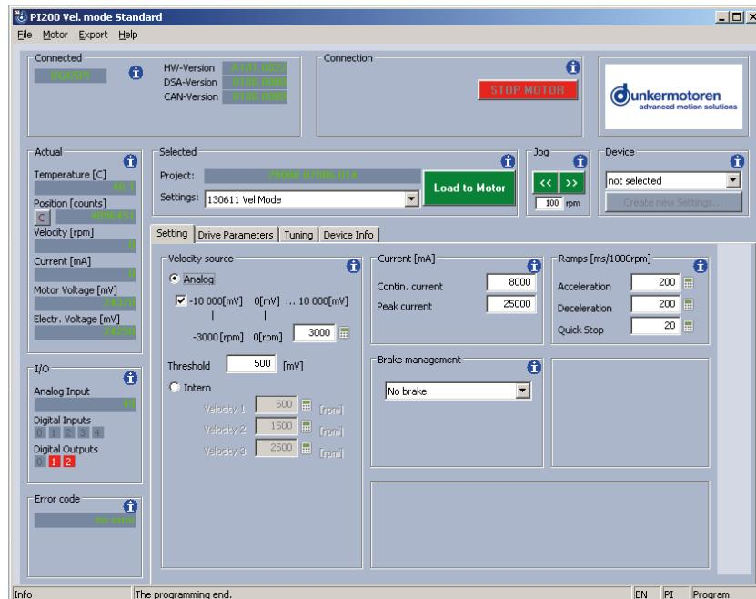
With the „Load to motor“ button, the user has the possibility of loading mode-specific parameter adjustments to the motor with the aid of the parameterising interface.
