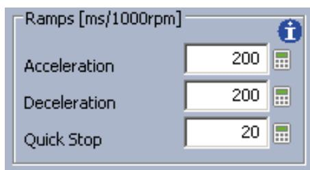
In this example, an acceleration ramp with 200 ms/1000rpm and a brake ramp with 200 ms/1000rpm were configured. For the Quick Stop, 20 ms/1000rpm was defined.
