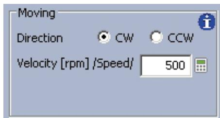
In this example, the motor runs with the speed of 500 rpm in the clockwise direction.
