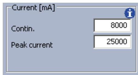
In this example, a continuous permissible phase current of 8 A and a peak current of 25 A are defined.
