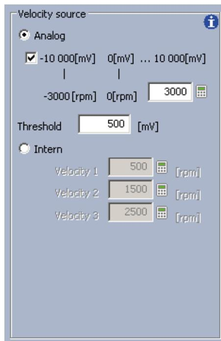
In this example, the velocity is regulated in an analog manner.
