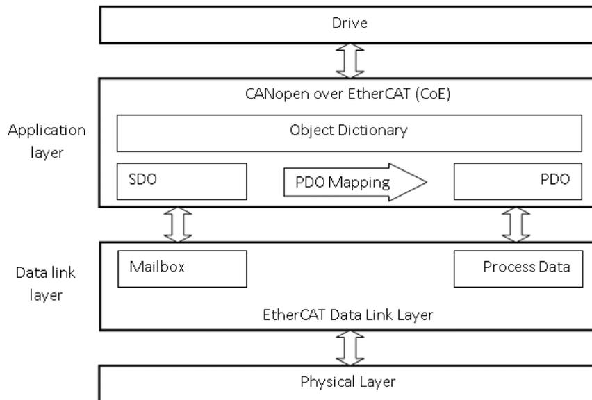
EtherCAT provides with the application layer “CANopen over EtherCAT (CoE)” the same communication mechanisms as the familiar CANopen mechanisms: object dictionary (drive parameters), PDO (process data objects) and SDO (service data objects) - even the network management is comparable. If you already used Dunkermotoren with CAN-bus interface, the transfer from CAN-Bus to CANopen over EtherCAT should be very easy.
