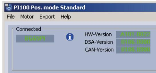
As long as the motor is not connected with the PC via the interface cable and the motor is not connected to the supply voltage, no version data are shown.
