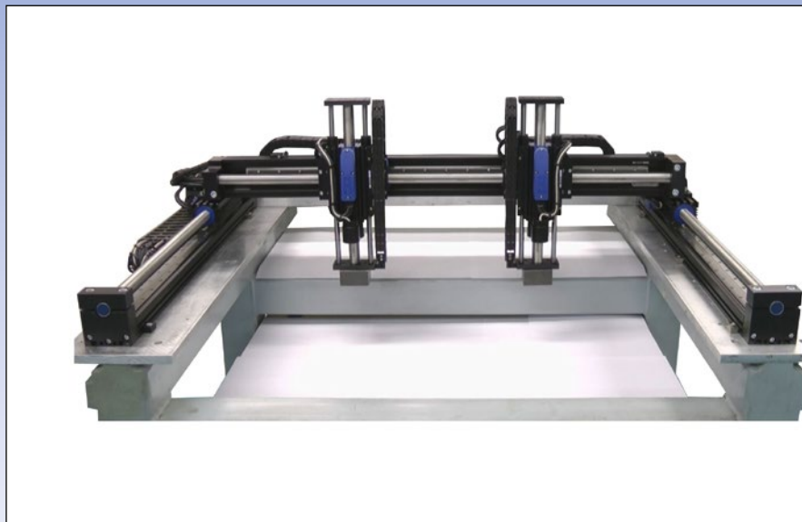
X, YY, ZZ multi-axis system with two independently moving Y/Z axes.
